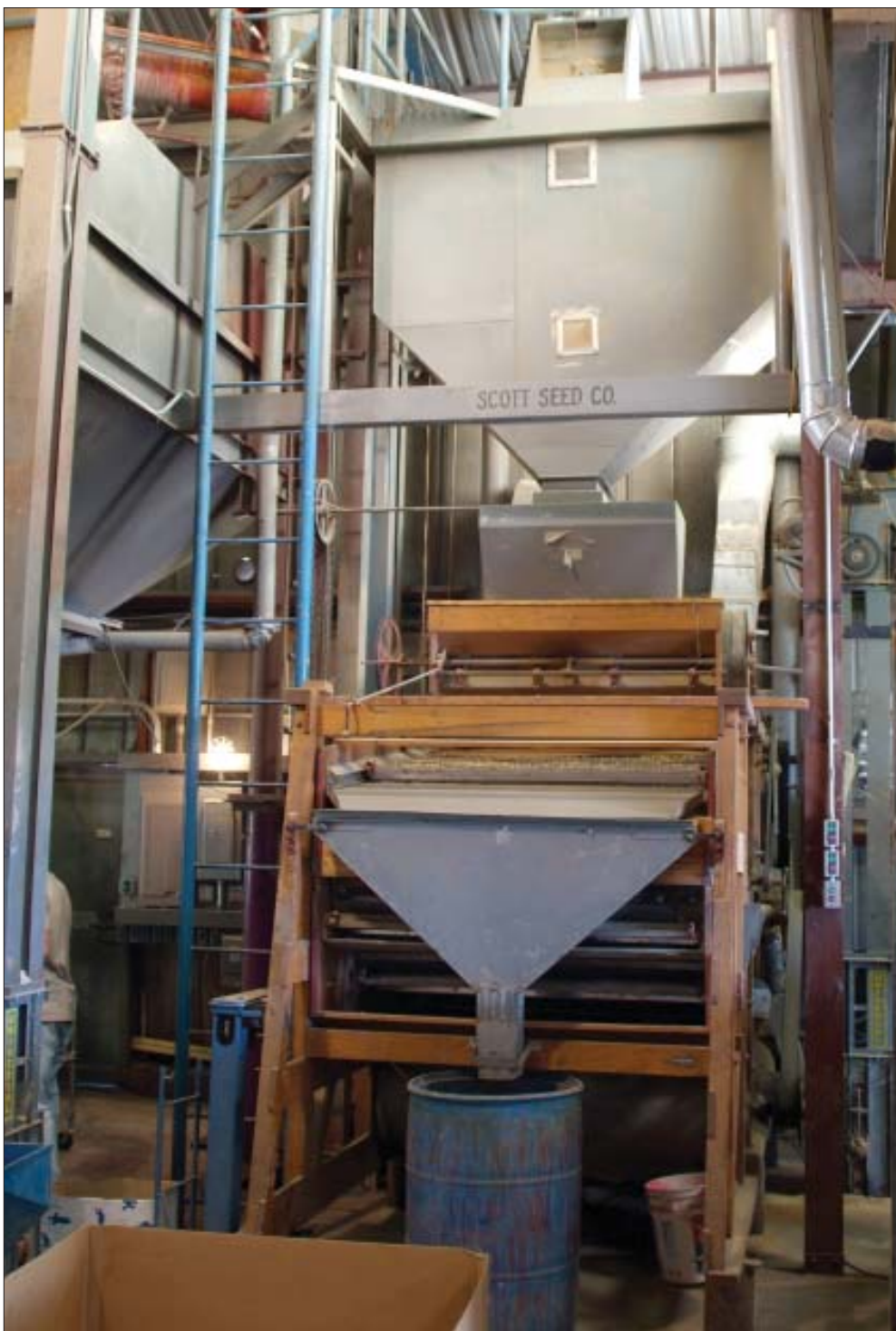
Scott Seed Company's sorghum seed is cleaned by a Clipper airscreen (right) and an Oliver gravity (not shown).
